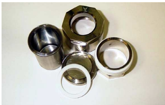
Fig. 2. Stainless steel container for PCT: vessel, lid, Teflon gasket, nickel-plated brass, nut, and screw.
